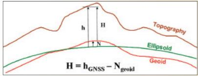
is determined by the difference between the ellipsoidal height (h), measured by GNSS, and the geoid height (N), interpolated from a geoid model. An orthometric height difference ( $\Delta$ H) can also be determined by levelling technique.
